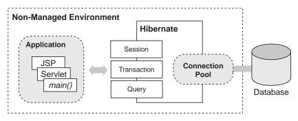
Figure 2.3 Hibernate with a connection pool in a non-managed environment
