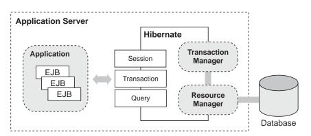
Figure 2.4 Hibernate in a managed environment with an application server
