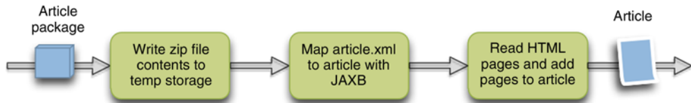
Figure 12.10 How ArticleConverter converts an article package to an Article
