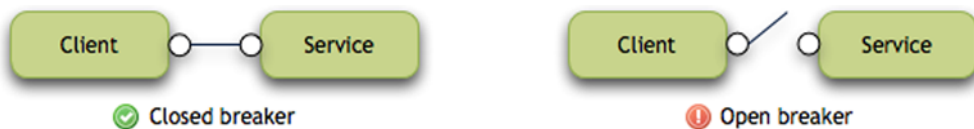
Figure 14.2 The breaker on the left is in the closed state, which is normal. Requests flow freely across a closed breaker. The breaker on the right is open. Requests can't flow across an open breaker.
